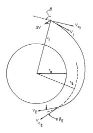
Fig. 1 Transfer orbit geometry (note: radii not to scale,  $\gamma_E$  defined at 400,000 ft)
