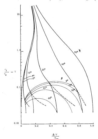
Fig. 2 Nondimensional retrofire impulse for deboost from circular orbit
