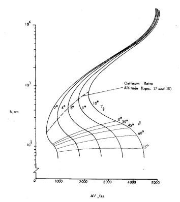
Fig. 3 Optimum retrofire altitude and retrofire angle for minimum  $\Delta V$
